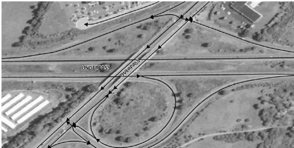
**Figure 2e:** Does not meet NENA and Virginia standard for elevated crossings. Arrows indicate endpoints; centerlines segmented at overpass and underpass
