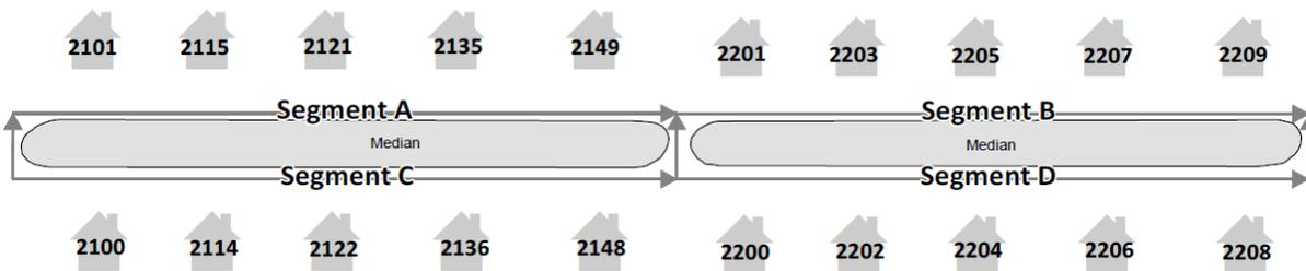
For dual carriageway centerlines, interior addresses are zeroed out on the left and right hand street side within the centerline depending on location because generally speaking, there are no physical addresses than can be located due to a physical barrier. Where barriers reside and dual carriageways are created within the centerline, interior address ranges are represented with a 0 range number from and to:
