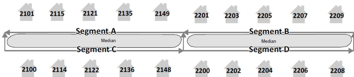
Where dual carriageways exist and using the RCL directionality standard, both sides of the median or barrier should be travelling in the same direction and addresses ranges should be zeroed out on the interior segment sides. Dual carriageway segments should be travelling with traffic flow on one side of the street and against traffic flow on the other while each segment should be attributed accordingly with the one way indicator field.
