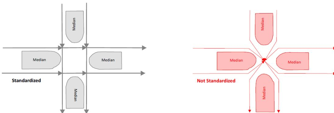
There are other combinations that can be made when working with dual carriageways and median segments as they meet other potential carriageway patterns. The included graphics are the most basic way to view the complexities and should be used when digitizing specific centerline intersection types.
