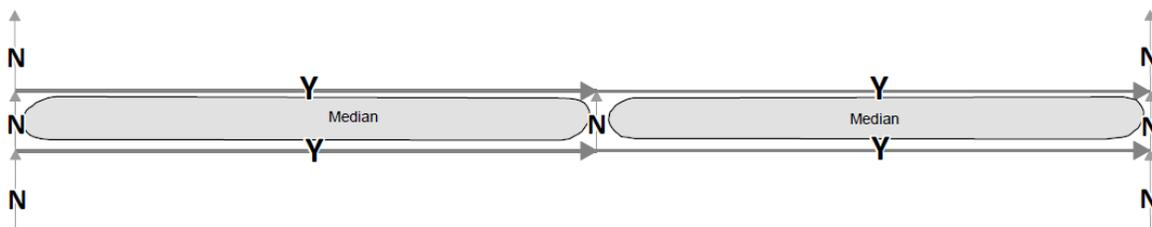
The VGIN RCL data model contains an indicator field for segments that are considered dual carriageway. This field makes analysis of road network ideal and also provides a good resource when performing QC to one way attribution within the data model along with address low and high fields.
